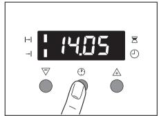
The function indicators Cook time  $\rightarrow$  and End time  $\rightarrow$  light up and the current time is shown in the display. In this case 12:05.
